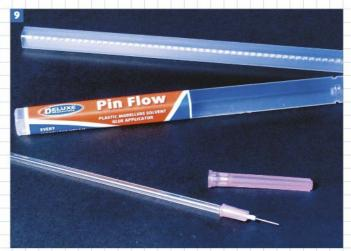
Hints and Tips: Always draw or pull the tip. If it becomes blocked then immerse in it glue overnight. Always replace cover when not in use and store in the outer case. Don't contaminate Plastic Magic bottles with a paintbrush as that might add plastic particles and clog the 'Pin Flow' tip
