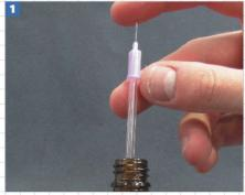
Drawing 'Plastic Magic' adhesive into the 'Pin Flow Applicator' is simple. Just invert the open end of the tube and place your clean finger over the 'Blunt' needle to retain the Plastic Magic in the tube. Then withdraw and invert to allow the glue to run down to the tip
